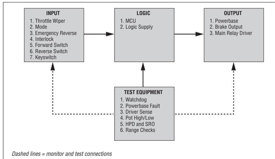
To mitigate the hazards typically found in machine operations, EN13849 requires that safety functions be defined; these must include all the input, logic, outputs, and power circuits that are involved in any potentially hazardous operation. Three safety functions are defined for the Curtis 1212S controller: (1) crushing due to unintended or uncontrolled movement; (2) crushing through loss of STO/braking; and (3) loss of stability from excessive speeds, as specified by vehicle limits.
