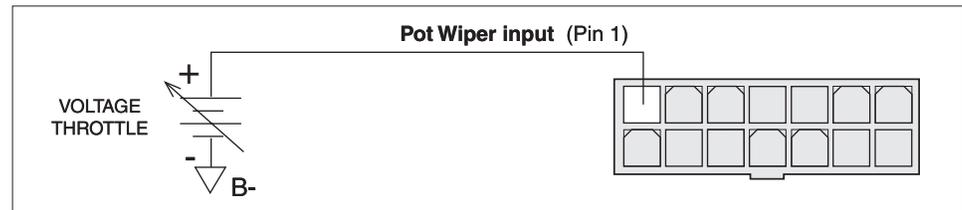
The PotHigh and PotLow parameters are used to set the voltage range of these throttles. If the pot wiper voltage is higher than the programmed PotHigh value or lower than the programmed PotLow value, the controller will issue an out-of-range throttle fault. In order for the controller to be able to detect out-of-range throttle faults, the throttle must have a range within the limits of 0.4–4.6 V.
