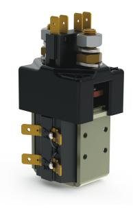
The SW80 has been designed for direct current loads, including motors as used on electric vehicles such as industrial trucks, and telecom and power distribution applications. Developed for both interrupted and uninterrupted loads, the SW80 is suitable for switching Resistive, Capacitive and Inductive loads.
