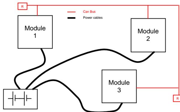
The red lines are can wires.
