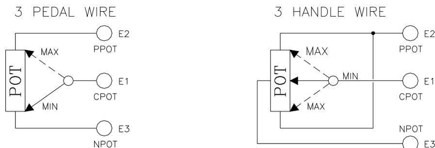
The Procedure for automatic potentiometer signal acquisition is carried out using the Console. This enables adjustment of the minimum and maximum useful signal level (PROGRAM VACC function), in either direction. This function is unique when it is necessary to compensate for asymmetry with the mechanical elements associated with the potentiometer, especially relating to the minimum level.
