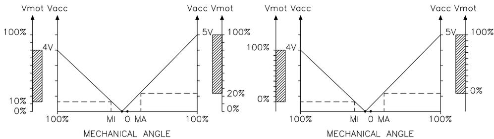
This function looks for and remembers the minimum and maximum potentiometer wiper voltage over the full mechanical range of the pedal. It enables compensation for non symmetry of the mechanical system between directions. The operation is performed by operating the pedal after entering the PROGRAM VACC function.
