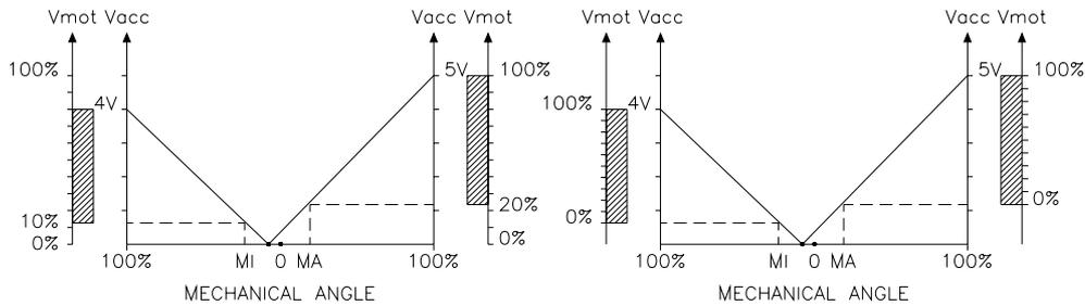
The two graphs show the output voltage from a non-calibrated potentiometer with respect to the mechanical “zero” of the control lever. MI and MA indicate the point where the direction switches close. 0 represents the mechanical zero of the rotation.
