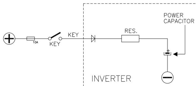
When the key is switched ON, the inverter tries to charge the capacitor through a power resistance, and check if the capacitor are charged within a timeout. If this is not true: an alarm is signalled; the main contactor is not closed.
