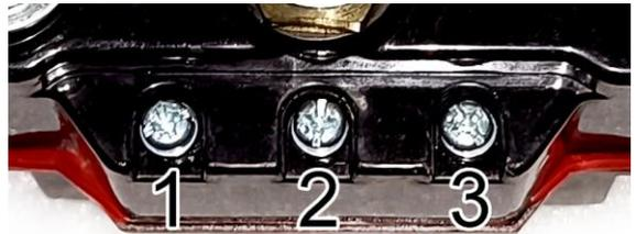
Coil connections are by means of 3mm screws
